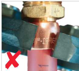
Jaw not square on the crimp ring
