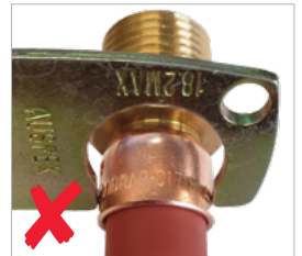
Fitting has been under crimped
