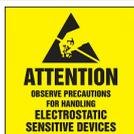
**CAUTION:** this product uses semiconductors that may be damaged by electrostatic discharges (ESD). When handling the printed circuit board, care must be taken not to damage the electronics.
