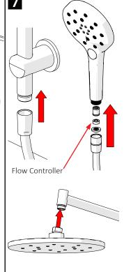
TEST AND CHECK FOR LEAKS.
