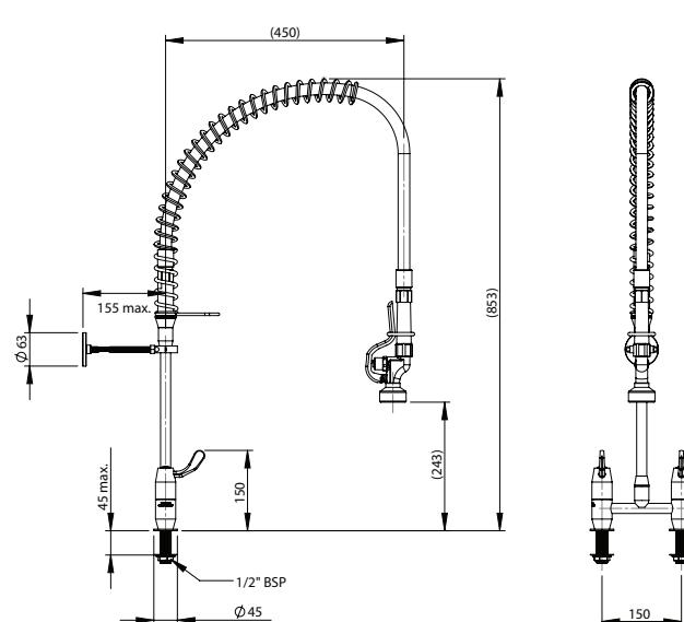
Spray gun position dimensions are approximate and represent a brand new unit, spring will sag with use over time
