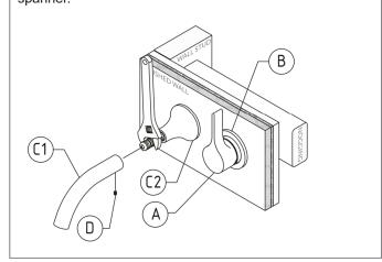
9) Fit the spout (C1) onto the post of the Flange (C2). Align and secure by tightening the set screw (G).
