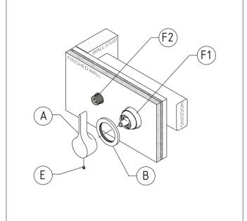
4) Ensure that the Handle (A) is fully engaged on the cartridge lever. Secure the handle by tightening the Set Screw (E) and Tighten well. The lever of the Handle (A) is to point up. Pulling the lever away from the wall will allow water flow.
