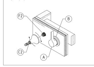
8) Tighten the Flange (C2) by hand and secure with a spanner.
