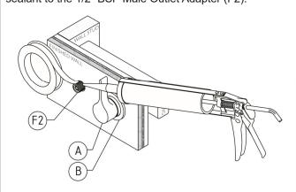
7) Screw the Flange (C2) onto the 1/2" BSP male outlet adapter (F2)
