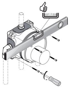
Use suitable supporting washers under the screw heads
