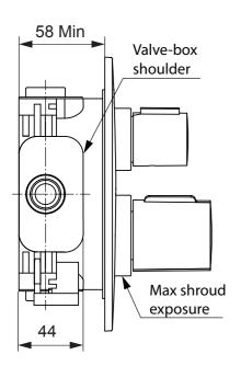
Cosmetically, when the escutcheon plate is furthest back (valve-box trimmed at MIN), this exposes more of the shroud diameters under the handle.
