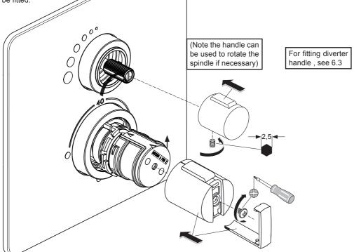
With the escutcheon in place, the flow control handle can be fitted. IMPORTANT: First rotate the black drive spline fully clockwise until it stops. Align the flow control handle to the 12'o-clock position (fin at top) & slide the handle onto the spindle & push firmly until it stops. The grub screw can be fitted from the underside of the handle using a 2.5mm hex key.
