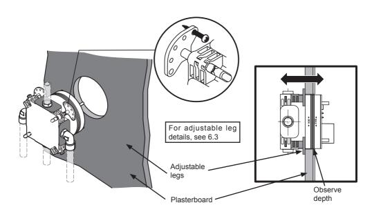
Mounting option C illustrated above using OPTIONAL adjustable fixing legs.
