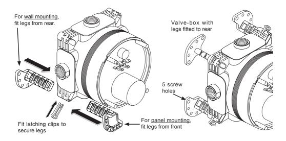
Note; If further depth adjustment is required, the latching clips can be easily be removed by pulling on the projecting lobe of the clip. Slide the leg along the slot until a more suitable leg-groove is visible, and then refit the latching clips to secure.
