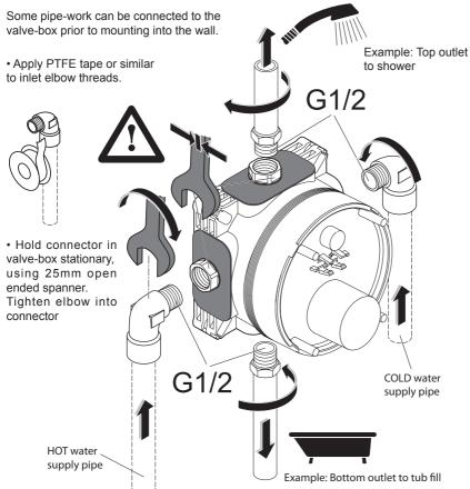
Alternatively, instead of PTFE tape, use an approved thread sealant; e.g.: Loctite 577 or Permabond A1044. DO NOT SOLDER NEAR VALVE-BOX.
