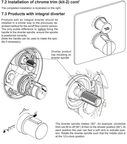
Orientate the diverter handle to the 12'o-clock position (fin at top) & slide the handle onto the spindle & push firmly until it stops. The grub screw can be fitted from the underside of the handle using a 2.5mm hex key.
