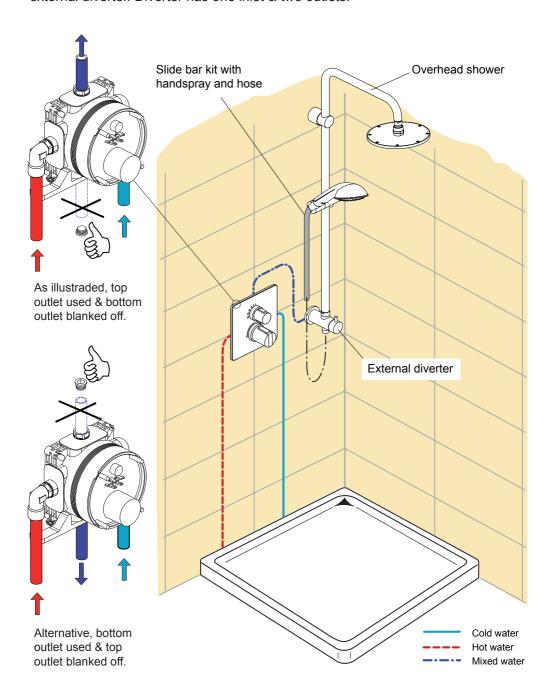
Three outlet example showing thermostatic shower valve with integrated "diverter" connected to a slide bar shower kit, overhead shower & body jets via an external diverter. Diverter has one inlet & two outlets.
