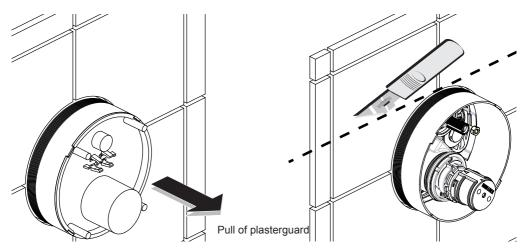
Illustrated above, valve-box projecting from the finished wall at the correct depth. The plaster guard can now be removed to expose the valve assembly inside.
