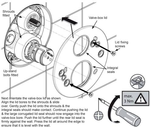
Insert the lid fixing screws into the countersunk holes in the lid as shown.
