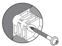
ADJUSTABLE LEGS OPTION (C) fit the OPTIONAL legs to the valve-box, from the front; to the desired depth (see 5.2C & 6.3). Guide the valve-box into the large hole, until the legs stop against the rear of the panel. Check level & valve-box orientation (see 5.4). Confirm valve-box is projecting from the front of the panel between the min & max depth markers (see 5.1). Adjust leg positions if necessary. Mount the valve-box to the panel using wood screws though the leg fixing holes
