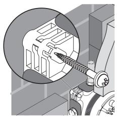
**A.** Directly through the valve-box using the 4 corner slots onto a solid surface. This method does not allow for any depth adjustment.
