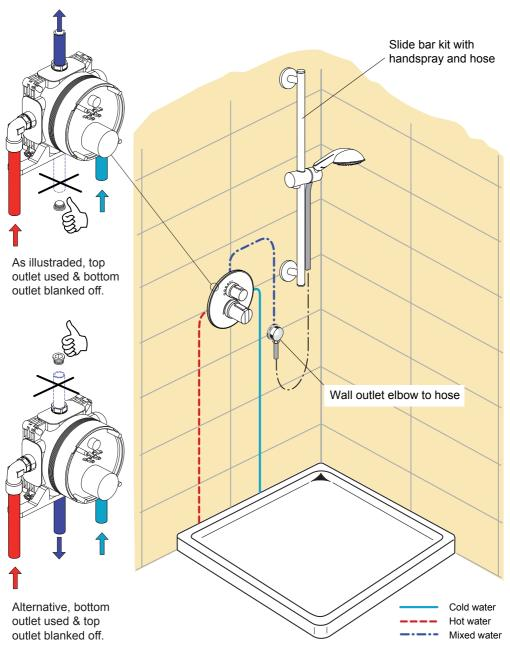
Two outlet example showing thermostatic shower valve with integrated "diverter" connected to slide bar shower kit & overhead shower.
