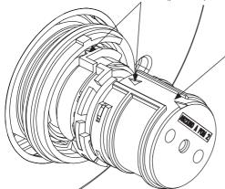
Orientate the temperature handle so that the button is at the top (as shown above). The location lug inside the handle should slide along the groove in the handle carrier. Push the handle along until it stops on the front face of the carrier.
