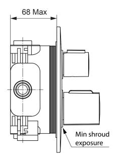
Conversely, when the escutcheon plate is furthest forward (valve-box trimmed at MAX), the shroud diameters under the handle are hardly noticeable.
