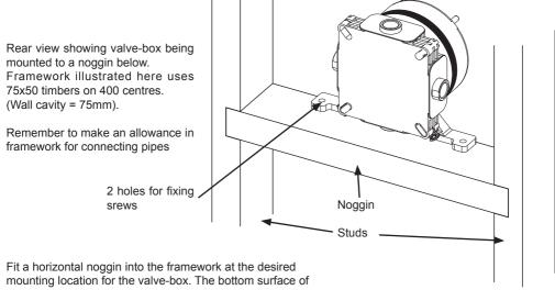
the bracket is 75mm from the centre of the valve-box. Therefore, the top edge of the noggin should be positioned 75mm below the desired valve-box centre. Ensure noggin is level & secured.
