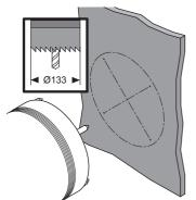
The large hole to be cut in the panel or plaster board should be Ø133mm (5.1/4"), which permits some clearance around the valve-box diameter (Ø129mm)
