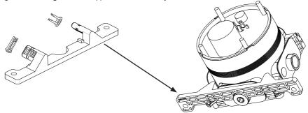
C. Using adjustable fixing legs (OPTIONAL) in either direction (x4 positions)
