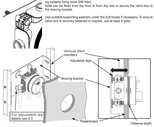
Mounting option C illustrated above using OPTIONAL adjustable fixing legs
