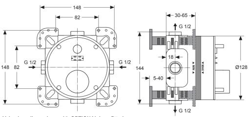
Valve-box dimensions with OPTIONAL legs fitted
