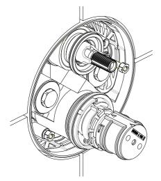
Illustrated on the left, the valve-box has been correctly trimmed. In this example, the product is the version with the integral "flow control".
