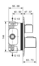
Inlets & Outlets are threaded G1/2". The escutcheon plate can float 10mm between min & max markers thus permitting mounting depth to vary.
