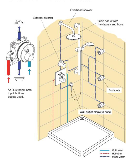
Three outlet example showing thermostatic shower valve with integrated "diverter" connected to a slide bar shower kit, overhead shower & tub fill. External diverter has one inlet & two outlets.
