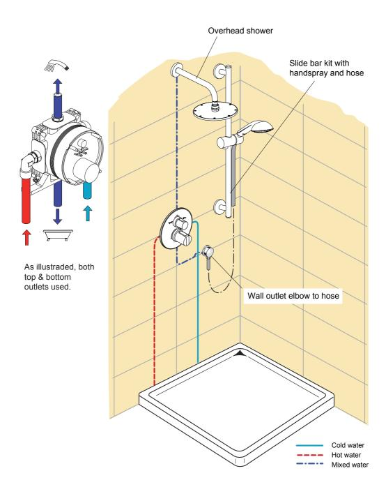
Two outlet example showing thermostatic shower valve with integrated "flow control" connected to a slide bar shower kit & overhead shower via external diverter. Diverter has one inlet & two outlets.
