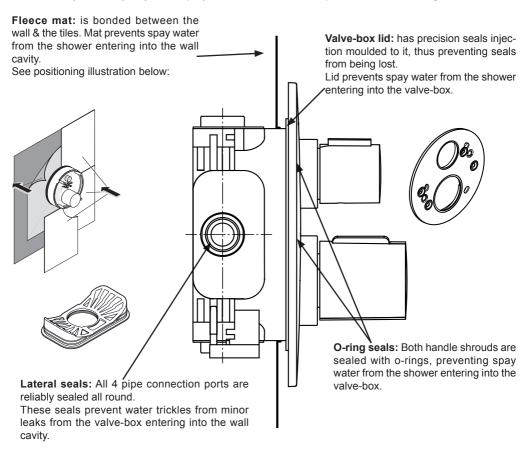
**Leak warning system:** In the event of a leak occurring inside the valve-box, the accumulated water will begin to drip from the gap between the temperature handle & the shroud. If a drip occurs, this indicates there is a problem & the chrome trim kit should be removed & the leak fixed. This leak path is designed to freely permit drainage of water from inside the valve-box into the wet area of the bathroom (but prevent water from escaping into the wall cavity).
