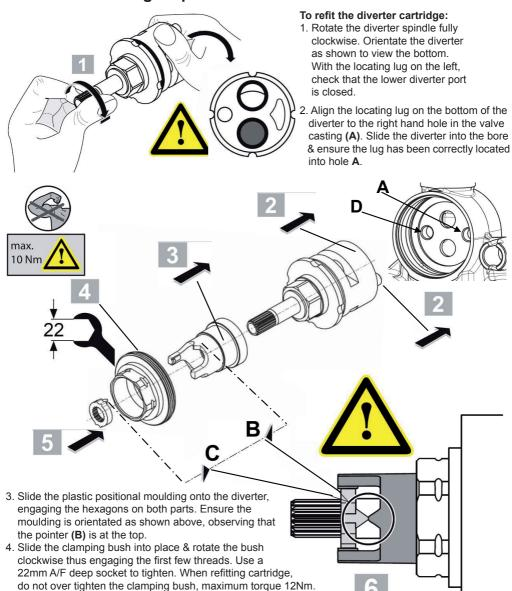
(C) is aligned to pointer (B). Both parts are splined, so the sleeve can be removed rotated & refitted until alignment is achieved. Once aligned, press the sleeve firmly. This will force the two lugs on the black moulding to move apart
