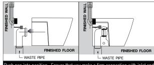
Push pan into position. Ensure that you make a firm connection with inlet and outlet pipes and avoid disturbing the floor fixing brackets. Flush test for leaks.
