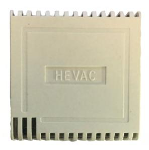
The SRTA-D is an averaging type room sensor to be used in pairs (wired in parallel). It is intended for use with Hevac brand HTC 3, 5 and Digital series controllers. The sensor has a NTC characteristic (increase in temperature = decrease in resistance) and changes approximately 160 ohms per degree.
