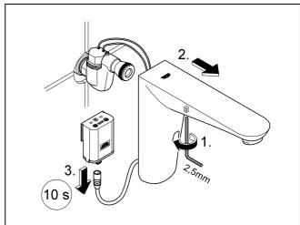
Disconnect the power supply to the electronics and re-connect after 10 s. Setting mode is active for 3 minutes.
