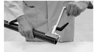
Chamfering the pipe
