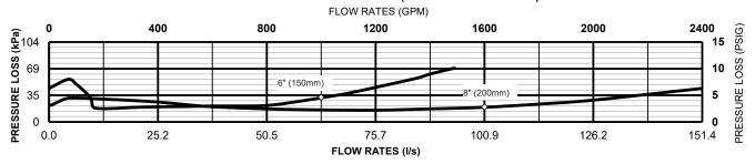
Note: The pressure losses depicted in the tables are for the device only and not the complete assembly.
