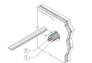
5) Unscrew Locknut (C) cut and Deburr prior to re-fitting onto spindle and tightening well.
