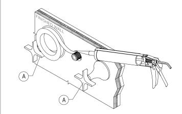
15) Screw the Flange (F2) onto the Wall Breech (1/2" BSP) until it meets the wall.
