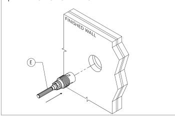
2) Once Fitted, Ensure both spindles (E) are set to OFF position - HOT = FULL TURN CLOCKWISE and COLD = FULL TURN ANTICLOCKWISE.
