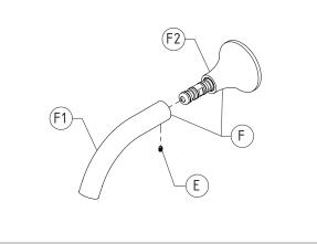
14) Ensure the area is clean and clear of debris. Seal the wall penetration and apply teflon tape or alternative sealant to the wall breech thread.
