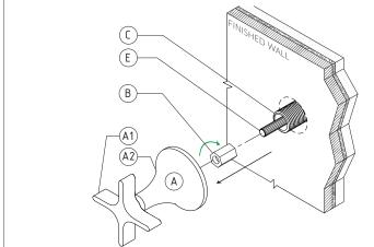
12) Re-fit Spindle Hex Adapter (B) and Handle Assembly (A) Repeat step 9-12 until horizontal handle alignment is achieved.
