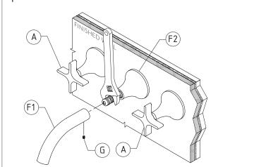
17) Fit the spout (F1) onto the post of the Flange (F2). Align and secure by tightening the set screw (G).
