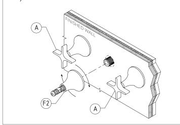
16) Tighten the Flange (F2) by hand and secure with a spanner.
