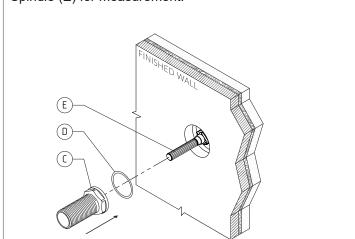
4) Measure the amount of Locknut (C) thread protruding from the finished wall and mark between **15-20mm**.
