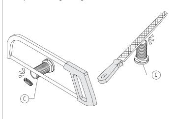
6) Measure Spindle length protruding from finished wall. This should measure between **25mm** and **30mm**. Cut if necessary.
