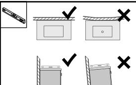
Ensure the wall is plumb and flat. If the vanity is fixed to a wall that is not flat or is out of plumb, there is a risk of drawer / door misalignment. The basin will also not sit level which may cause water to pool.
