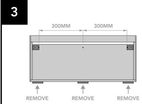
Securely fasten the vanity to the wall using appropriate fasteners. Secure the cabinet to the wall through the top left and right hand brackets. Ensure fixings are no less than 300mm apart. Fixings at the bottom of the cabinet should be no more than 100mm from each end of the cabinet and no more than 50mm from the base panel.
