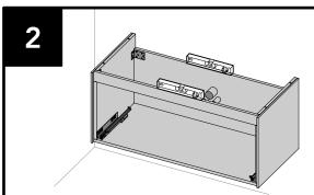
Position the vanity in the correct location and fix with a single central screw into the support beam. Ensure the vanity is completely level.
