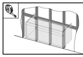
Wall hung vanities and basins must be securely attached to wall studs. If necessary, install additional support noggins at desired locations prior to sheeting the wall
