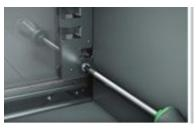
Half turn 1x screw to unlock the height adjustment.
