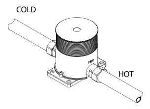
5. Make sure the concealed box is perfectly horizontal and then lock it up with expansion screws.
