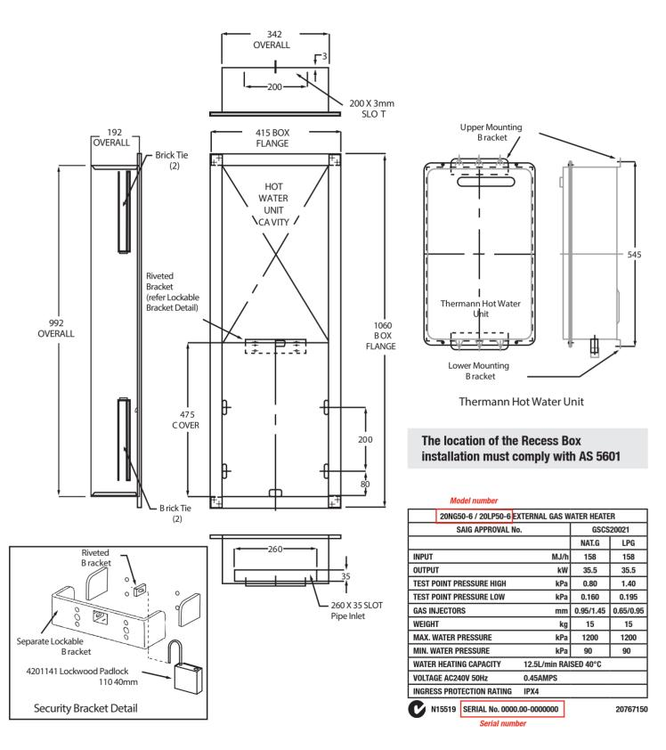
NOTE: Before installing your hot water unit, copy the serial number and model number information from the rating label located on the side of the water heater to the inside page of the *Thermann Installation manual* for future reference.
