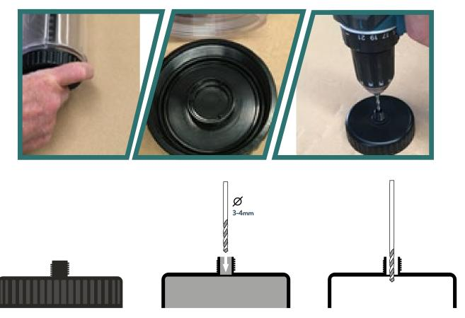
Unscrew the cleaning cap by hand, place the cap on a flat surface and carefully drill a 3-4mm hole as shown
