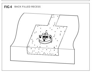
\* To install this floormount fixing valve, a 50mm step down (recess) is required in the concrete slab. The floormount fixing valve is supplied with end caps, pressure plate and fixing bolts. Leave intact until final fit off with the floormount mixer.
