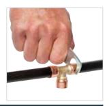
If the gauge experiences any interference the joint is under crimped. The tool should then be adjusted. (See adjustment instructions in this manual). Do not double crimp.
