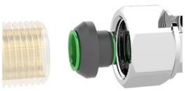
Installation is easy and quick. **Thread** the loose nut connection to the threaded pipe with your hand (no tooling is required), leave it not too tight, ensure that the valve can rotate axially. **Adjusts** the valve in the correct orientation. Once located at your convenience, **tighten** the loose nut preferably using a spanner. Do not over tight the loose nut to avoid cutting the cone washer.
