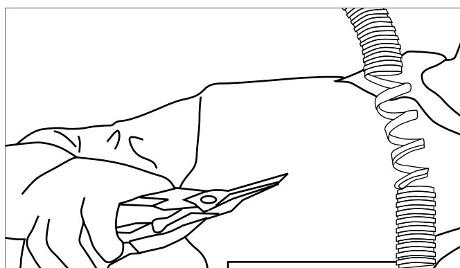
Fig. A2-5 Cutting of RAUGUARD
