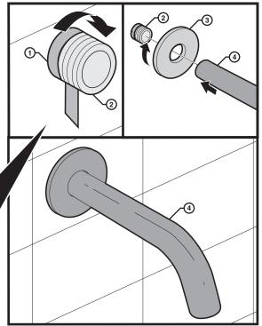
Note: Basin Outlet is pre-fitted with a 5 Star rated WELS Aerator. For Bath applications, Outlet Aerator must be changed to the supplied Bath Aerator packaged in the box.
