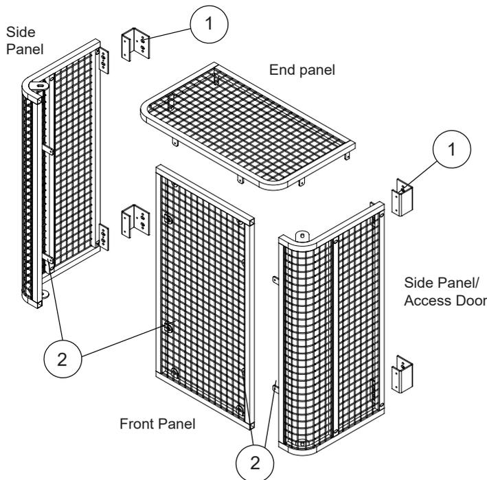
1. Join mounting brackets to side panel with M6 x12.
