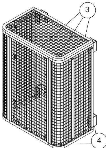
3. Fit end panel and secure with M6 x12 (2) and M6 x30 (4).
