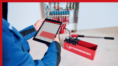
Wireless readout of the test data via Bluetooth®
