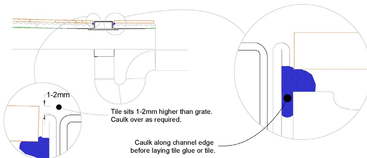
Ensure the channel is completely level
