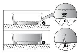
4. Using the appropriate silicone for the surface type, apply a thick bead of silicone within the bath outline.
