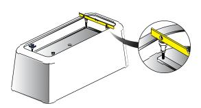
2. Check that bath sits flat; if required adjust legs to compensate for floor level.
