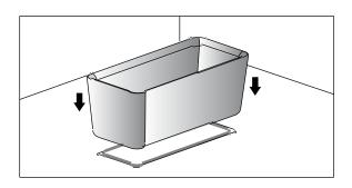
3. Ensure waste connection is set in position. Placing the bath in position, pencil the outline. Connect waste and test for leakages and drainage.
