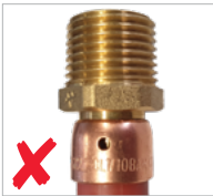
Witness hole not completely filled
