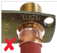
Fitting has been under crimped
