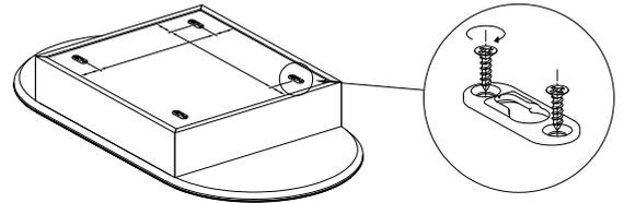
2. Drill pilot holes in cabinet to line up with pre-determined timber support located in the wall.
