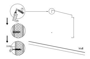
**3.** Fix cabinet to wall using appropriate screws for the relevant wall material. Take care not to over tighten screws.
