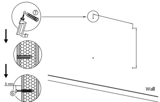
3. Fix cabinet to wall using appropriate screws for the relevant wall material. Take care not to over tighten screws.
