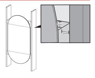
5. Ensure the cabinet carcass protrudes by a minimum of 20mm from the wall (including tiles) to allow for finger pull on the door.
