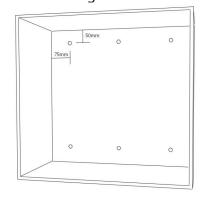
The number of fittings used to fix cabinet will depend on the size of unit, your installer will know the suitable amount depending on the size of your cabinet.
