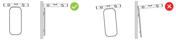
5. Hook mirror to the wall mounted bracket, you can also use silicone to mount the mirror permanently.
