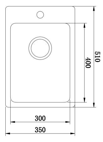
Please note that cutout template is provided as a guide only. This cutout template should be checked against actual sink unit to determine correct fit. 490mm
