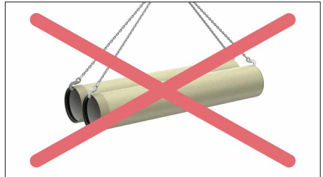
Fig. 3: Hooks and wire ropes must not be used in direct contact with the pipe for transportation
