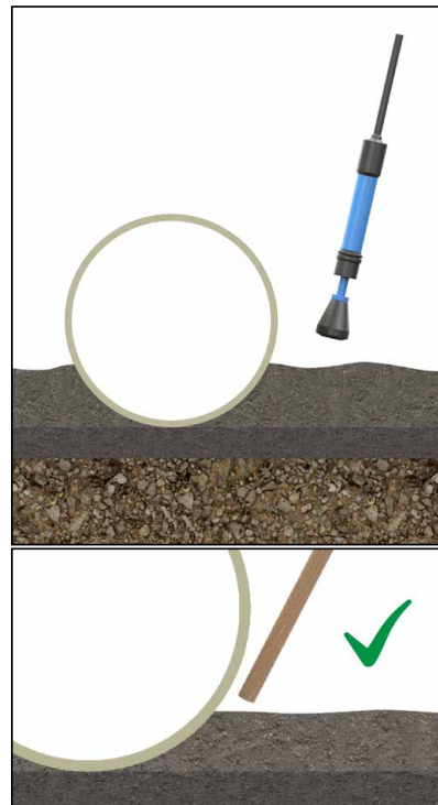
Fig. 15: Proper haunch backfill
