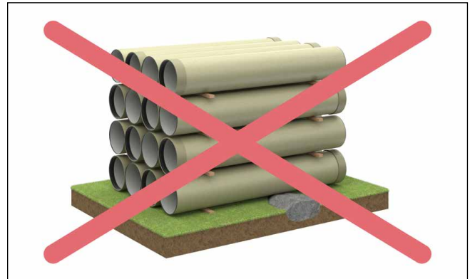
Fig. 8: Pipes should not rest on stones
