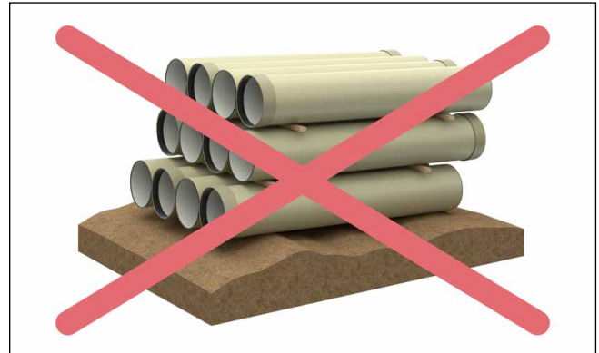
Fig. 9: Pipes should not rest on an uneven surface
