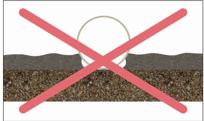
Fig. 14: Improper haunch backfill
