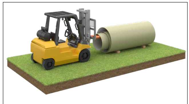
Fig. 5: Denesting of pipes with protected forks
