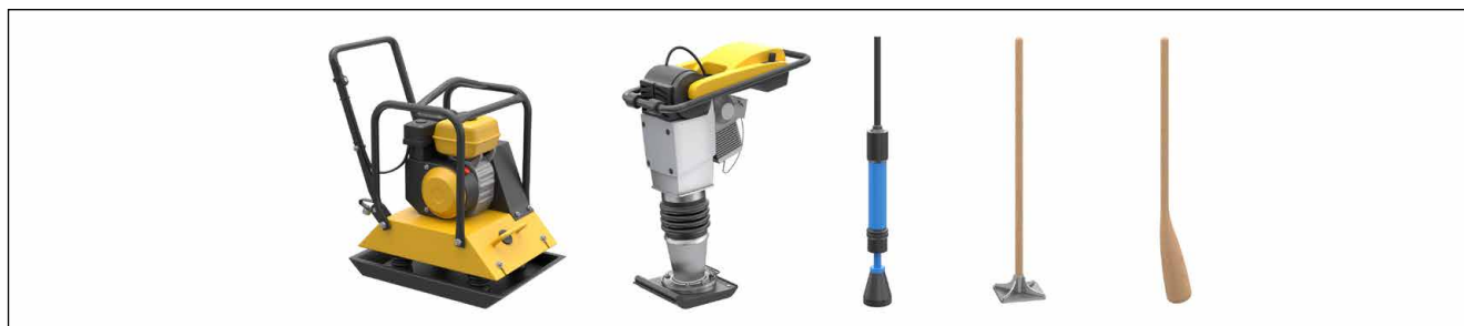
Fig. 19: Hand-operated compaction equipment
