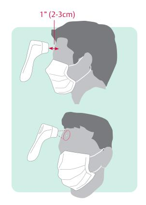
For accurate temperature readings ensure the thermometer is held at the distance shown above.
