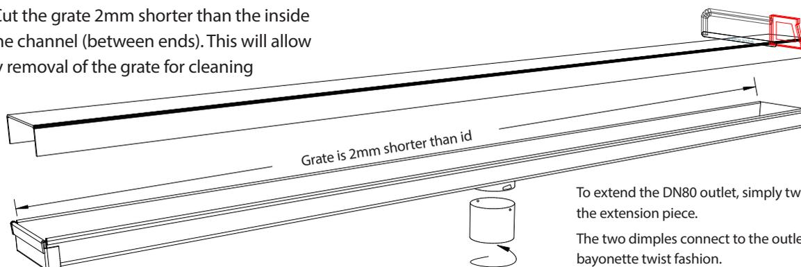
To extend the DN80 outlet, simply twist on the extension piece.
