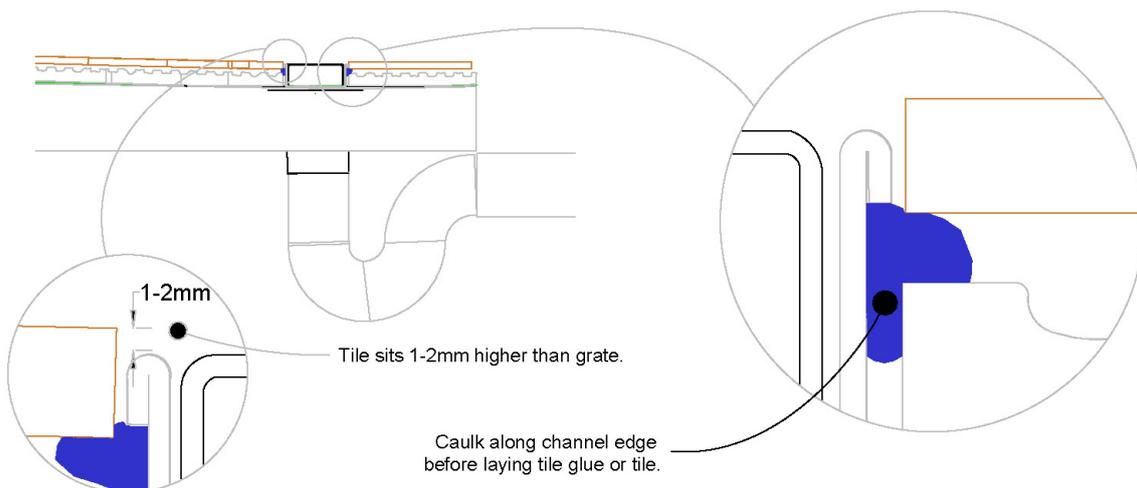
Ensure the channel is completely level
