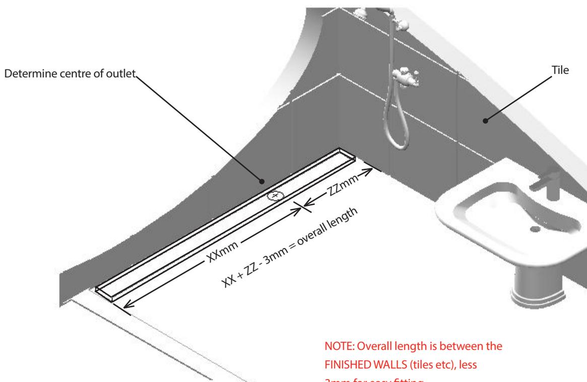
**NOTE:** Overall length is between the FINISHED WALLS (tiles etc), less 3mm for easy fitting.
