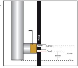
Place Towel Rail in correct position over mounted brackets, secure unit in place by tightening grub screw on inside of each bracket arm with Alan key provided. Fig 3. and Fig 4.
