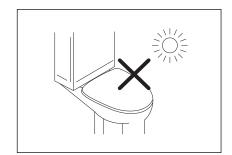
The closing speed of the seat with slow close function can vary with the changing of room temperature and use cycles.
