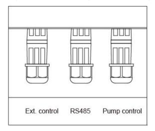
**Warning:** Above connections are suitable only for use with extra-low voltage. Mains power supply connection must not be made to the connectors.
