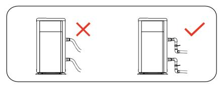
Use only pressure PVC or equivalent plastic pipes that are capable of withstanding the pressure and temperature expected from the pool system and the heat pump.
