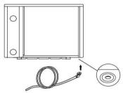
c. Run the drain hose to an appropriate discharge point while maintaining a continuous fall.
