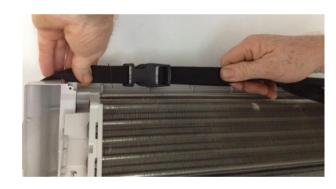
Adjust the strap to hold the bag in position.
