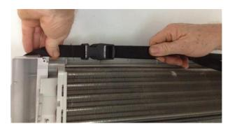
Place the strapping over the exposed evaporator coil.
