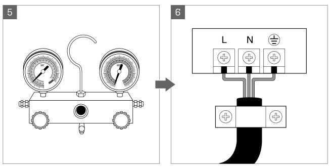
Leak test and evacuate the refrigeration system (Page 26)
