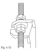
Mount the indoor unit onto the hanging screw bolts with a block. Position the indoor unit flat using a level indicator to prevent leaks. (See Fig. 4.9).
