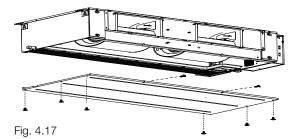
• Loosen the four bolts and two screws which are used to fasten the front side plate (be careful, the front side plate may fall down).
