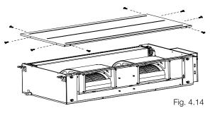
• Loosen the four bolts and two screws which are used to fasten the front side plate.
