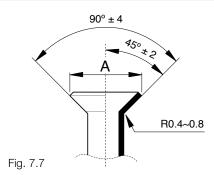
Remove the flaring tool and flare form, then inspect the end of the pipe for cracks and even flaring.
