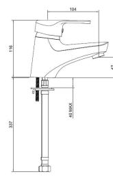
CONSTRUCTION: Brass body CARTRIDGE TYPE: Ceramic CLASSIFICATION: Suitable for all pressures INLET CONNECTIONS: 1/2 " BSP WORKING PRESSURE: 35 - 500kPa DIMENSIONS FOR FITTING: 35mm diameter hole OPERATING TEMPERATURE: 5 °C - 65 °C
