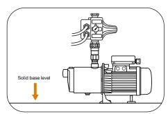
**Note:** If you are installing the VFB-APC directly onto the Horizontal Multistage Pump, use a 25mm barrel union. If you are installing the VFB-APC between the pump and first outlet, use pipework with a minimum internal diameter of 25mm.
