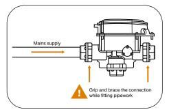
**Note:** Brace this fitting to prevent movement while connecting to the mains supply.
