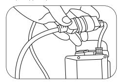
Connect the power lead to the power outlet. Do not turn on.
