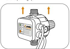
Check the set up so far. Ensure that the VFB-APC is braced or fixed so minimal movement occurs once in operation. If the distance between the pump and highest outlet exceeds 15m, adjust the cut-in pressure on the VFB-APC.
