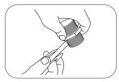
Thread the nipple into the female socket of the pump discharge until it is watertight. Do not overtighten.
