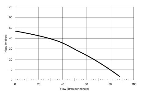
Note: The curve above represents the pump with the VFB-APC.
