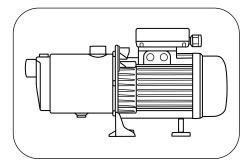
**Note:** It is recommended the pump should be no further than 3 metres from the tank.
