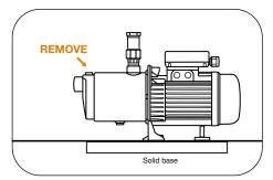
Slowly fill the pump casing and suction line with water through the priming port (best done with a funnel) allowing air to vent as the water fills the suction line and pump casing. If there are any leaks, repair these immediately. If no leaks are present, proceed.
