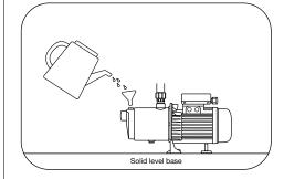
4. Once the suction line and pump casing are full of water and all air is expelled, replace the priming port plug. Your pump is now primed. Before pump operation ensure there is sufficient water inside the tank.
