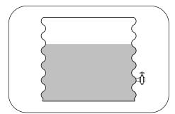
Open the isolation valve on the tank. If there are any leaks, repair these immediately.
