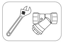
Use a steel brush to clean the dirt from the filter.
