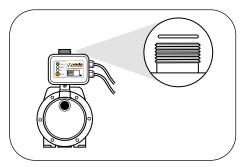
Hold the Mechanical Switching Unit (VFB-MSU25) over the outlet and connect the loose nut. Do not overtighten. The rubber washer will lock this in place.
