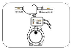
For easy maintenance down the track, install an isolation valve into both the mains and house water line.
