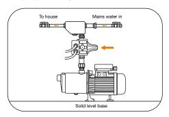
Using a flat head screwdriver, turn the adjustment screw clockwise until you reach the correct pressure (roughly, this will be 3.5 full 360° turns).
