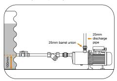
**Note:** It is crucial that you use the recommended pipe size until at least the first pipe branch (T piece) is reached.
