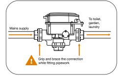
For easy maintenance install an isolation valve on either side of the VFB-DSU.
