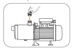
Connect the 25mm female end of the barrel union to the nipple until it is watertight. Do not overtighten.
