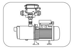
7. Connect the 25mm female end of the switching unit to the incoming mains water supply. This is marked 'MAINS' with an arrow pointing out of the VFB-DSU (indicating water flow direction).
