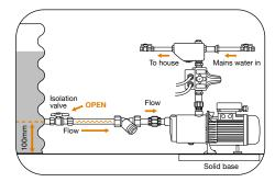
2. Slowly open the gate valve on the discharge line to 50%.
