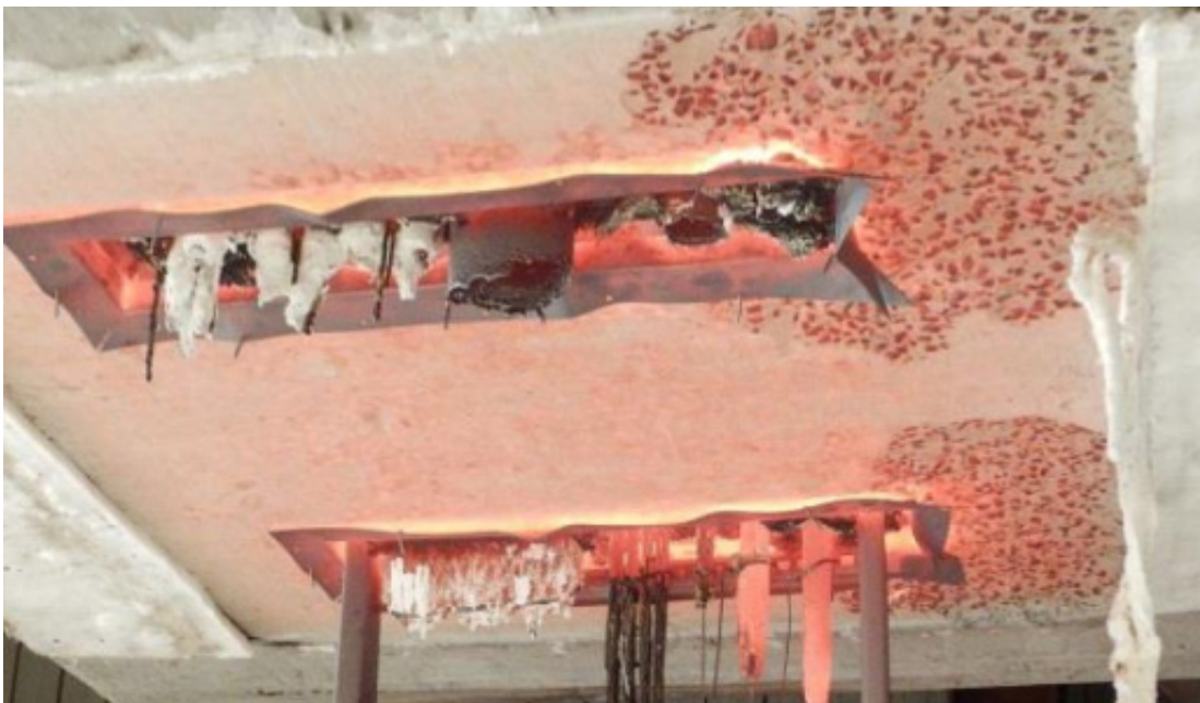
FyreBOX™ Cast-In after a 4 hour test.
