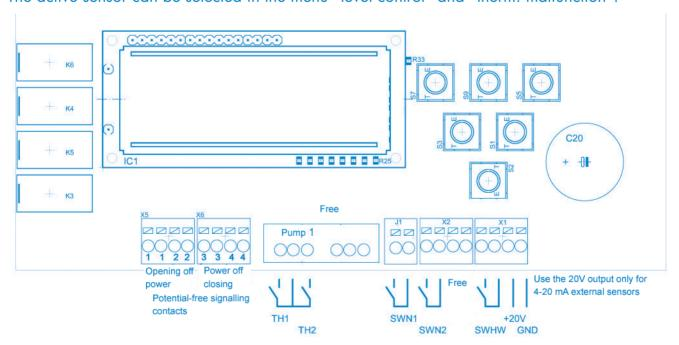
If the thermostatic switch TH2 is not necessary, a bridge has to be inserted on this contact point. The thermostatic switch TH1 can be deactivated via the menu therm. malfunction.
