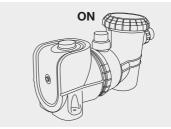
Check there are no water leaks 2 and verify adequate flow to and from the pool.
