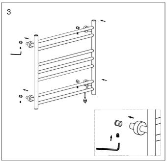
• With the allen key provided, tighten the grub screws to ensure that towel rail stays in position.
