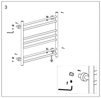
• With the allen key provided, tighten the grub screws to ensure that towel rail stays in position.
