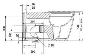
Note: All measurements should be taken from the finished wall/floor
