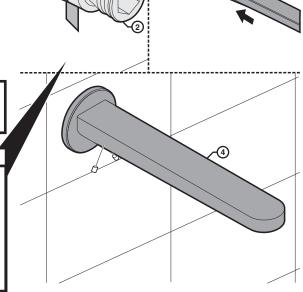
Note: Basin Outlet is pre-fitted with a 6 Star rated WELS Aerator. For Bath applications, Outlet Aerator must be changed to the supplied Bath Aerator packaged in the box.
