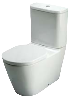
Back to Wall Toilet Suite WELS: 4 star, 4.5/3 ltr/flush Average flush: 3.3 litres Standard and Soft Close seat available S Trap: 140-270mm P Trap: 190mm
