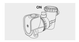
Check there are no water leaks and verify adequate flow to and from the pool.
