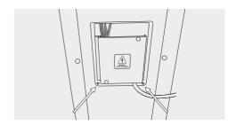
Once removed, you will see the High Voltage protective cover. Using a Phillips head screwdriver remove the two screws.
